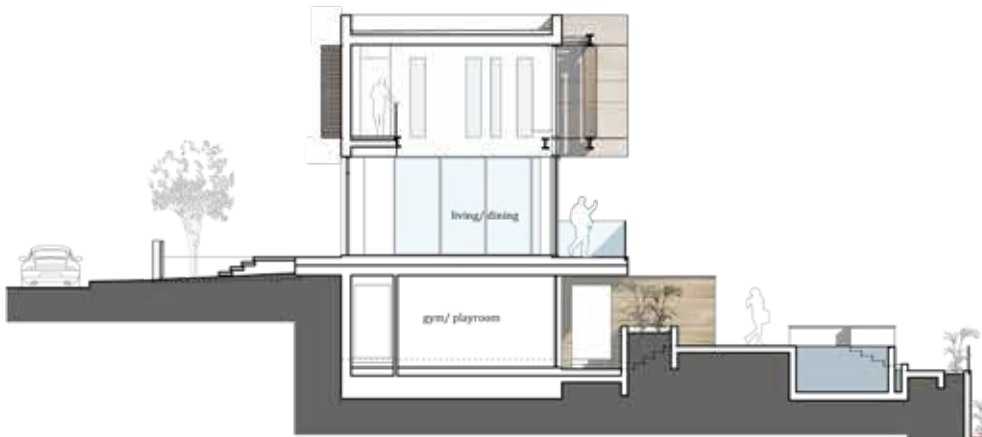
Section a-a (West Elevation) Villa A
